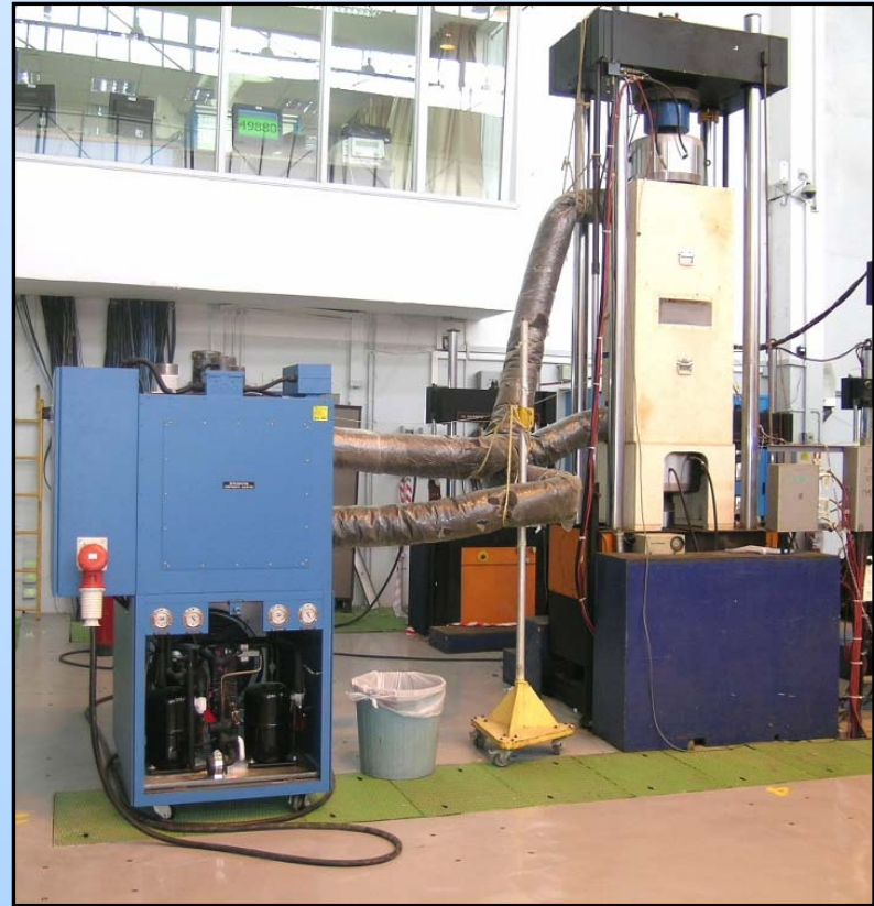
Test Setup for the Carbon-Epoxy Reinforced Panel tested at -50°C
